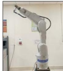
Six Axis Articulated Robot Manipulator
